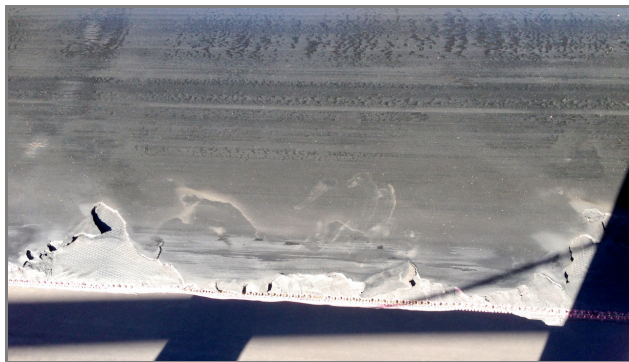
The edge damage to the fabric belt
