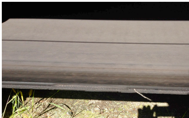
The edge damage to the fabric belt
