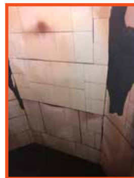
CoBond's Solution - 6 months after install and 8M tonnes of Iron Ore
