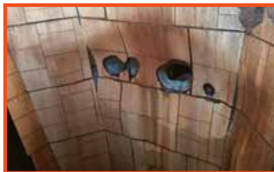
Competitors Solution - 7 months after install and 9.5M tonnes of Iron Ore
